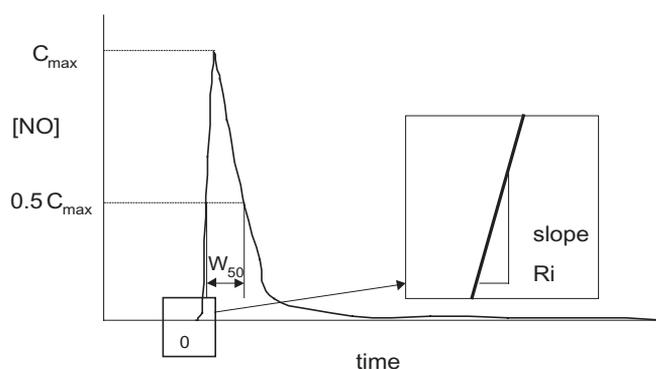
Figure 2. Schematic of the indices characterizing NO release kinetics: peak concentration ( $C_{\text{max}}$ ), window of time the concentration exceeds 50% of the maximum ( $W_{50}$ ), and initial release rate ( $R_i$ ).
