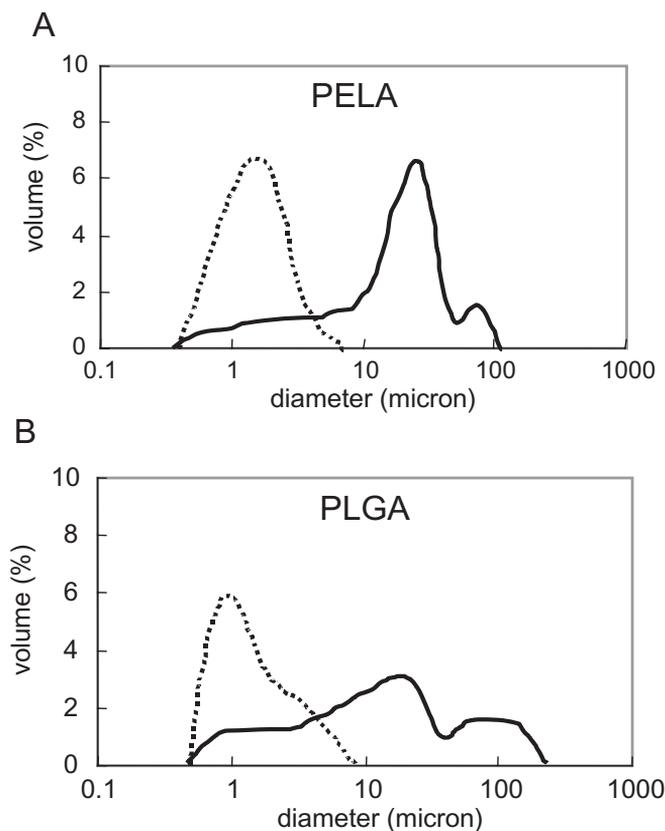
Figure 4. Size distribution profile of microparticles containing PROLI/NO in the presence (solid line) and absence (dashed line) of gelatin. (A) PELA-based (5% PEG); (B) PLGA-based.
